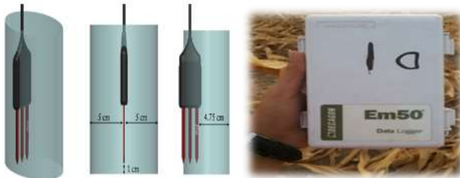
Figure 1. Mechanism for placing sensors in the soil.
